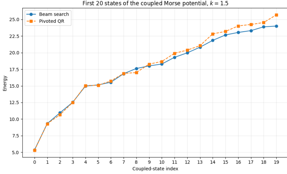
Figure 10: First 20 energies for the coupled Morse potential with k = 1.5 using the beam-search and pivoted-QR point sets. The plot quantifies the sensitivity of the nonseparable calculation to the collocation-point selection.
